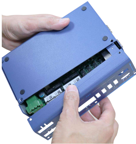
Remove front IO panel
