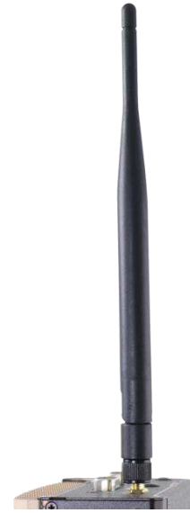
Attach external antenna
