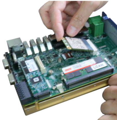
Insert on a 45 degree angle
