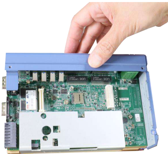
Remove front IO panel
