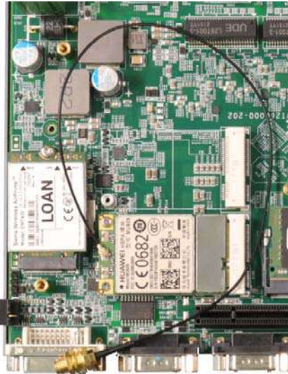
Clip on the IPEX-to-SMA cable
