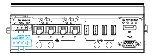
The "Remote On/ Off" 3-pin connection allows for external switch extension. It is useful when the system is placed in a cabinet or a not easily accessed location. You may connect an external remote with an external status LED indicator (15mA) by connecting to PWR LED and GND.
