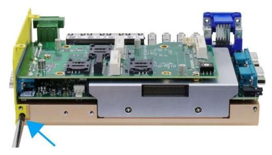
2. Install the front panel by securing it with three screws and two hex-bolt screws on the VGA connector.
