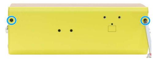
4. Turn the system upside-down, remove the three screws indicated and separate the L-shape enclosure panel from the heatsink/ mainboard.
