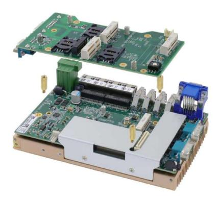
4. Then secure the  $\mathsf{MezIO}^\mathsf{TM}$  module to the hex bolts with three (3) P-head screws.
