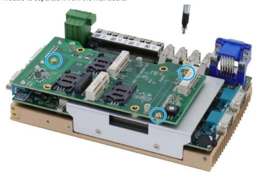
Remove the two screws shown below and remove the heatsink covering the DRAM module and M.2 slot.
