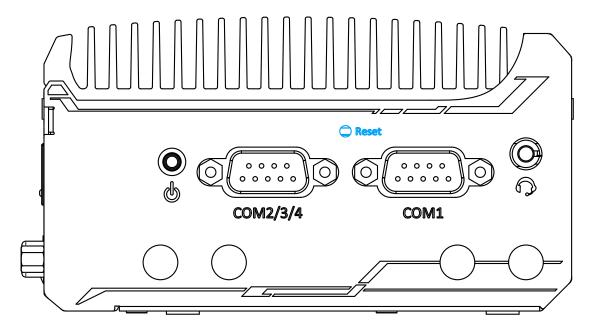
The reset button is used to manually reset the system in case of system halt or malfunction. To avoid unexpected reset, the button is purposely placed behind the panel. To reset, please use a pin-like object (eg. tip of a pen) to access the reset button.
