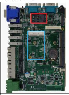
mini-PCle/ SIM slot on the MezIO™ module
