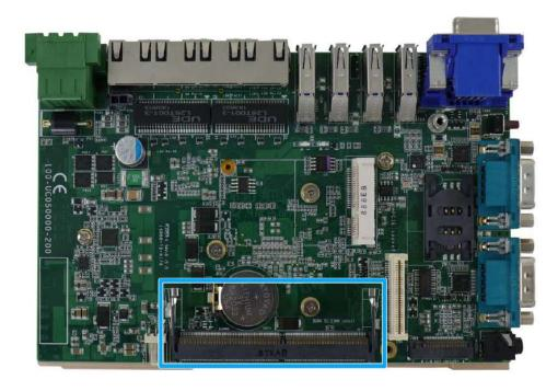
3. **To install**, insert the gold finger end of the SO-DIMM on a 45 degree angle into the slot and gently push the SO-DIMM down until it is clipped-in.
