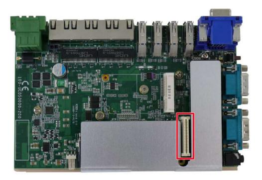
2. Remove the screws indicated in red and replace with stand-off hex bolt screws.
