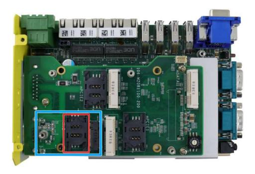
3. To insert a SIM card, push and flip the slide-and-clamp slot towards the center of the  $MezIO^{TM}$  module.
