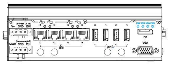
There are four LED indicators on the front panel: IGN, WDT, HDD and PWR. The descriptions of these four LEDs are listed in the following table.
