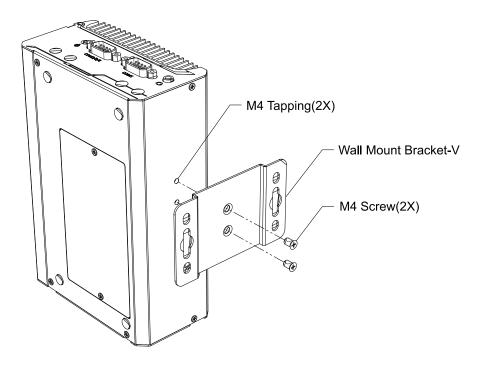
2. Dimension illustration of the install vertical wall mount bracket for your reference.
