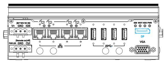
The system has a DisplayPort (DP) output which is a digital display interface that mainly connect video source and carry audio to a display device. When connecting a DP, it can deliver up to 4K UHD (4096 x 2160 @ 30Hz) in resolution. The system is designed to support passive DP adapter/ cable. You can connect to other display devices using DP-to-HDMI cable or DP-to-DVI cable.
