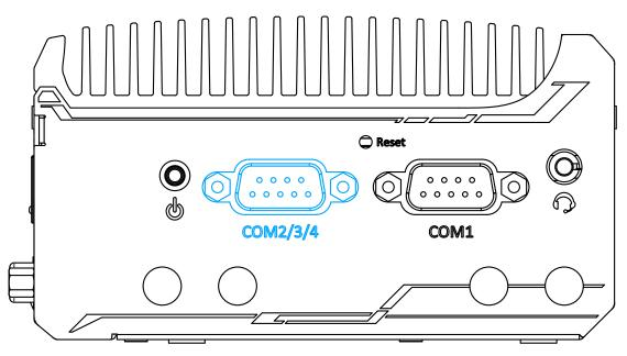
Implemented using industrial-grade ITE8786 Super IO chip (-40 to 85°C) and provide up to 921600 bps baud rate, the D-Sub male connector (COM2/ 3/ 4) can be configured in the BIOS as single RS-422/ 485 port (COM2) or three 3-wire RS-232 ports (COM2/COM3/COM4). Please refer to COM2/ 3/ 4 Port Configuration for configuring operation mode. An optional 1-to-3 Y-cable is available to connect three RS-232 devices.
