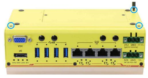
4. Secure the two screws to complete the enclosure.
