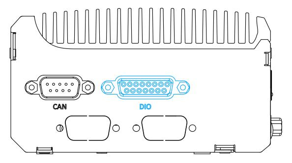
The system provides 4x isolated digital input channels and 4x isolated digital output channels. The DIO functions support polling mode I/O access and DI change-of-state interrupt. Please refer to <a href="Watchdog Timer & Isolated DIO">Watchdog Timer & Isolated DIO</a> for information on wiring and programming the isolated DIO channels.
