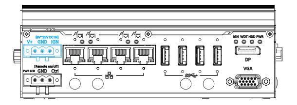
The system accepts a wide range of DC power input from 8 to 35V via a 3-pin pluggable terminal block, which is fit for field usage where DC power is usually provided. The screw clamping mechanism on the terminal block offers connection reliability when wiring DC power.
