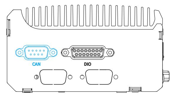
CAN bus is a robust industrial bus with a pair of differential signals and is commonly used in various industrial and in-vehicles applications. The system is equipped with a CAN bus DB9 port that is compatible with both industrial and in-vehicle applications. The CAN bus port supports CAN2.0A and CAN2.0B up to 1Mbps.
