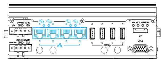
The Gigabit Power over Ethernet (PoE) port supply power and data on a standard CAT-5/ CAT-6 Ethernet cable. Acting as a PSE (Power Sourcing Equipment), compliant with IEEE 802.3at, each port delivers up to 25W to a Powered Device (PD). PoE automatically detects and determine if the connected device is PoE PD or not before supplying power, making it compatible with standard Ethernet devices as well.
