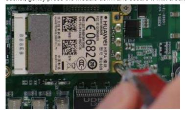
7. Clip-on mini-PCle module's antenna (please refer to the module's user manual on antenna cable connection).
