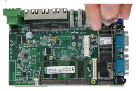
Once you have installed the NVMe SSD, you need to reinstall the heat spreader but before you do so, please make sure the protective film on the thermal pads have been removed.
