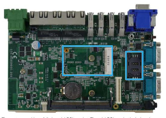
The system provides a full-size mini-PCIe socket. The mini-PCIe socket is designed with SIM card support. With a SIM card installed, your system can access the internet via your network provider's 3G/4G network.
