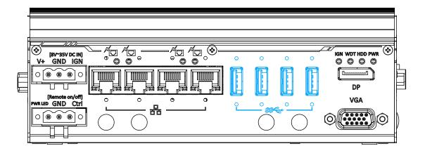
The system offers four USB 3.1 Gen1 (SuperSpeed USB) ports on its front panel. They are backward compatible with USB 2.0, USB 1.1 and USB 1.0 devices. Legacy USB support is also provided so you can use USB keyboard/mouse in DOS environment while USB 3.1 Gen1 driver is supported natively in Windows 10.
