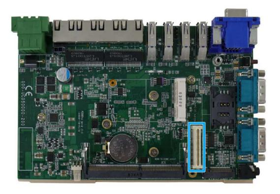
MezIO<sup>TM</sup> is an innovative interface designed for integrating application-oriented I/O functions into an embedded system. It offers computer signals, power rails and control signals via a high-speed connector. MezIO<sup>TM</sup> is also mechanically reliable benefited from its 3-point mounted mezzanine structure. A MezIO<sup>TM</sup> module can leverage these signals to implement comprehensive I/O functions.
