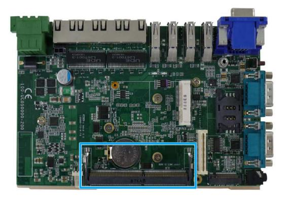
The system supports one 260-pin SO-DIMM socket for installing DDR4-2400MHz memory module up to 16GB in capacity.
