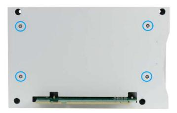
5. Disconnect the 2x 5-pin 2.0mm pitch cable from the connector, remove the screw securing the PB-2500J bracket, gently wiggle and lift PB-2500J out of the PCIe slot.
