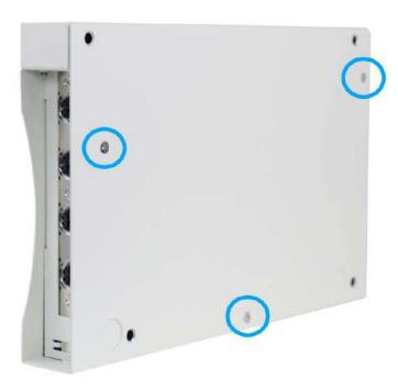
6. Gently lower the Cassette module back onto the system enclosure and secure the module onto the system enclosure by securing the following screws.
