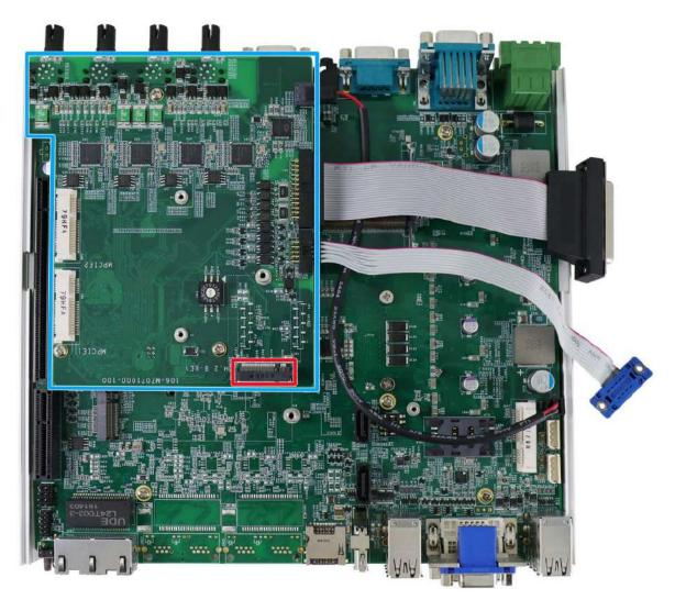
There is an additional M.2 2242 slot available on the MezIO<sup>TM</sup> module. To expand wireless networking capability, users can install off-the-shelf 3G/4G mini-PCIe modules and access the internet via the provider's network.
