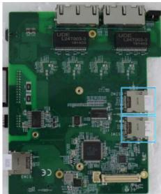
SIM slots underneath the mini-PCle slots on MezlO<sup>™</sup> module
