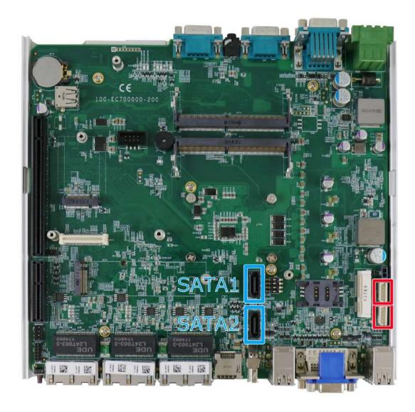
The system provides two SATA ports which support Gen3, 6 Gb/s SATA signals. Each SATA port (indicated in blue) features a 7-pin SATA connector and a 4-pin power connector (indicated in red).
