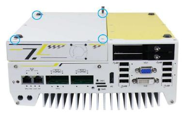
2. Gently wiggle the Cassette module and separate it from the system enclosure.
