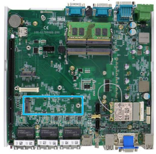
The system has a x4 PCIe M.2 2280 slot for you to install an NVMe SSD for the ultimate performance or an Intel® Optane<sup>TM</sup> memory to accelerate the read/ write performances of traditional hard disk drive. An NVMe SSD offers exceptional performance over 2.5" SSDs while Intel® Optane<sup>TM</sup> memory can dramatically boost your traditional hard disk drives' read/ write performances. For installation, please refer to the following instructions.
