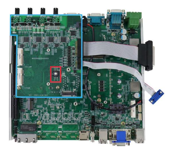
For Nuvo-7100/ 7200/ 7250VTC systems, the ignition control switch can be found within the enclosure, on the MezIO<sup>TM</sup> module. The ignition power control switch features multiple modes for pre and post ignition settings. Please refer to the section <a href="Ignition-Power Control">Ignition</a> <a href="Power Control">Power Control</a> for details.
