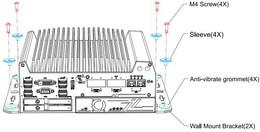
3. When wall mounting, place the heatsink fins perpendicular to the ground for better heat dissipation efficiency.
