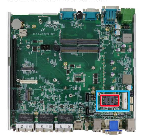
The system provides a dual mode mSATA/ mini-PCIe socket (indicated in blue) that is in compliance with mini-PCIe specification rev. 1.2. You can install either an mSATA SSD or mini-PCIe module into this socket and the system will automatically detect and configure it to run PCIe or SATA signals. This mini-PCIe socket is designed with SIM card (slot indicated in red) support. With a SIM card installed, your system can access the internet via your network provider's 3G/4G network.
