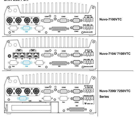
CAN bus is a robust industrial bus with a pair of differential signals and is commonly used in various industrial and in-vehicles applications. The system is equipped with a CAN bus DB9 port that is compatible with both industrial and in-vehicle applications. The CAN bus port supports CAN2.0A and CAN2.0B up to 1Mbps.
