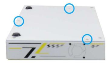
4. Turn the Cassette module to the connector side and remove the four screws.
