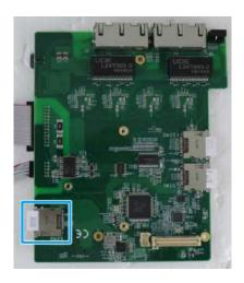
SIM slot underneath the M.2 slot on MezIO<sup>™</sup> module
