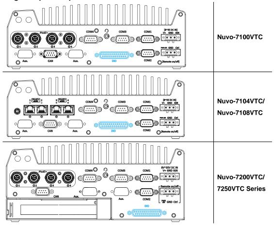
The system provides 4x isolated digital input channels and 4x isolated digital output channels. The DIO functions support polling mode I/O access and DI change-of-state interrupt. Please refer to digital I/O pin definition on the following page and <a href="Watchdog">Watchdog</a> <a href="Timer & Isolated DIO">Timer & Isolated DIO</a> for information on wiring and programming the isolated DIO channels.
