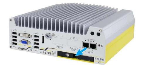
3. With the label side facing upward, insert the SATA connector side of the 2.5" HDD/ SSD into the slot first. You may feel resistance when the SATA connectors meet, push it in firmly until the 2.5" HDD/ SSD is fully inserted into the slot.
