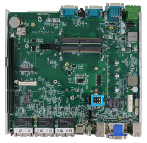
The DIP switch (indicated in **blue**) should be already configured out of the factory. Users need only set the 4th DIP switch to ON for BIOS update and switch it back to the OFF position when BIOS upgrade has completed. The table below shows the system default DIP switch settings for reference purposes.
