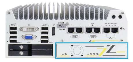
The Cassette module provides a separated compartment to accommodate an add-on card. It compartmentalizes the heat generated and effectively manages thermal conditions of both the system and add-on card(s). The modular design reduces the complexity of installing and replacing add-on card to offer system stability and reliability. To install a PCIe card into the Cassette module, please refer to the following procedure:
