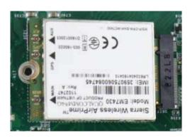
4. Gently press down and secure the module with an M2.5 P-head screw.
