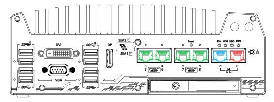
All Nuvo-7000VTC systems two GbE ports (in **red** and **blue**) while Nuvo-7108/ 7258VTC systems have four additional PoE (Power over Ethernet) ports marked in **green** on the front panel. All Ethernet ports feature panel screw fix holes for a firm connection. The port marked in **blue** is implemented using Intel<sup>®</sup> I219-LM controller that supports
