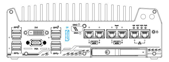
The system has a DisplayPort (DP) output which is a digital display interface that mainly connect video source and carry audio to a display device. When connecting a DP, it can deliver up to 4K UHD (4096 x 2304) in resolution. The system is designed to support passive DP adapter/ cable. You can connect to other display devices using DP-to-HDMI cable or DP-to-DVI cable.
