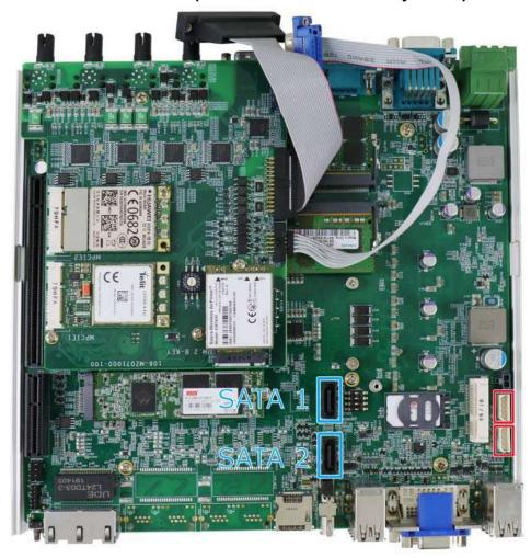
The system has two SATA ports (indicated in blue) and two four pin power connectors (indicated in red). The SATA and power cables should already be connected on the motherboard so users only need to install the HDD/ SSD. Please refer to the following instructions on how to install 2.5" SATA HDD/SSD.
