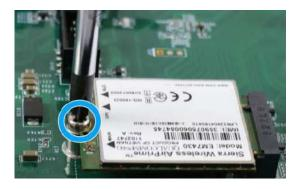
5. Clip on the IPEZ-to-SMA cable to the module and secure the antenna to the front or rear panel. Please refer to the module's manual for clip-on connection.
