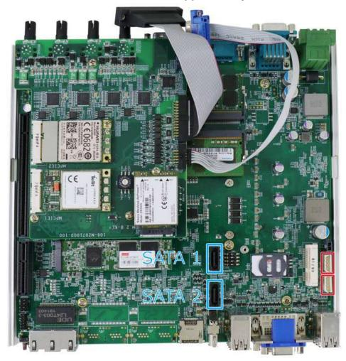
The system has two SATA ports (blue) and two four pin power connectors (red). The SATA and power cables should already be connected on the motherboard so users only need to install the 2.5" SATA HDDs/ SSDs to the front hot-swappable tray(s) For Nuvo-7100VTC systems, there is also an internal drive that can be coupled to configured into RAID 0 or 1 storage.
