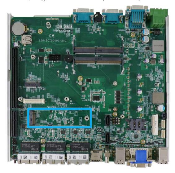
The system has an x4 PCIe M.2 2280 slot (also in compliance with SATA signal) for you to install an NVMe SSD for the ultimate performance or an Intel® Optane<sup>TM</sup> memory to accelerate the read/ write performances of traditional hard disk drive. An NVMe SSD offers exceptional performance over 2.5" SSDs while Intel® Optane<sup>TM</sup> memory can dramatically boost your traditional hard disk drives' read/ write performances.
