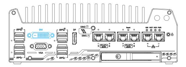
DVI-D transmits graphics data in digital format and therefore can deliver better image quality at high resolution. The DVI connector on the front panel can either output DVI signals or other digital signals (via an adapter/ cable) depending on the display device connected. It supports resolutions up to 1920x1200@60Hz.
