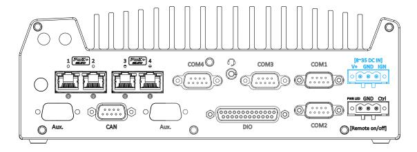
The system accepts a wide range of DC power input from 8 to 35V via a 3-pin pluggable terminal block, which is fit for field usage where DC power is usually provided. The screw clamping mechanism on the terminal block offers connection reliability when wiring DC power.
