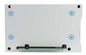
10. Secure the Cassette module cover by securing the three screws.
