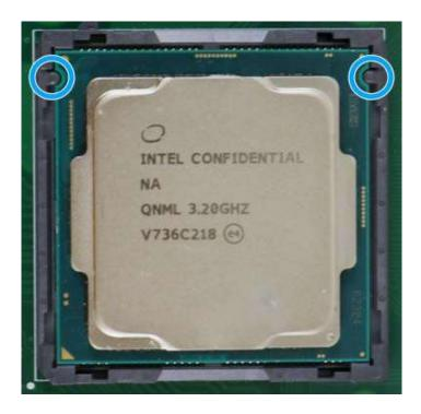
Locate the CPU retention bracket from the accessory box. Place the retention bracket on the CPU and hold it in place.
