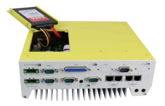
5. Gently put the tray back into the system with the connector side being inserted into the system first and secure the tray with three screws.
