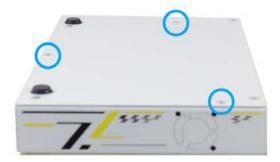
Lower the Cassette module onto the system and secure it with the four screws indicated.
