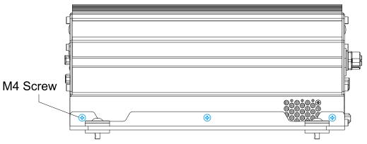
2. Place the system on a flat surface, insert the sleeves into the anti-vibration grommets and secure it with M4 screws.
