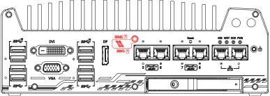
The system has an M.2 2242 slot (indicated in **blue**) that works with dual SIM slots (4G + 3G) on the front panel (indicated in **red**). By installing a 3G or 4G M.2 module and SIM card, you can access the internet via the provider's network.
