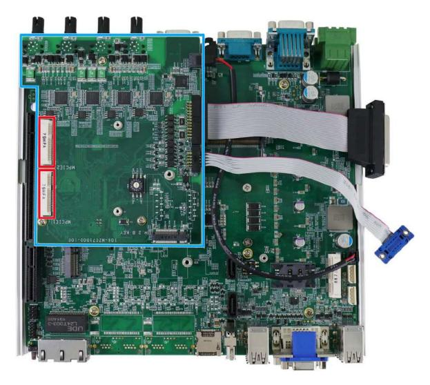
There are two additional full-size mini-PCIe sockets available on the MezIO<sup>TM</sup> module. They are implemented with USB signals only have better compatibility with off-the-shelf 3G/4G mini-PCIe modules. For customers who want to install 3G/4G module(s), please take advantage of these two mini-PCIe sockets and the associated SIM slots.
