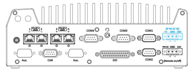
To have ignition power control for in-vehicle usage, you need to supply IGN signal to the system. The IGN input is located on the 3-pin pluggable terminal block (shared with DC power input). For in-vehicle ignition control wiring, please do the following:
