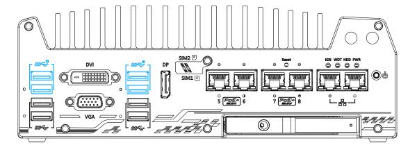
The system's USB 3.0 Gen 1 ports (5Gbps) are implemented via native xHCI (eXtensible Host Controller Interface) controller and are backward compatible with USB 2.0, USB 1.1 and USB 1.0 devices. Legacy USB is also supported so you can use USB keyboard/mouse in DOS environment
