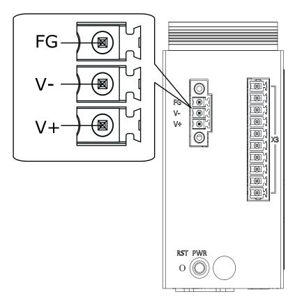
The DC connector can be located at the top of the system.
