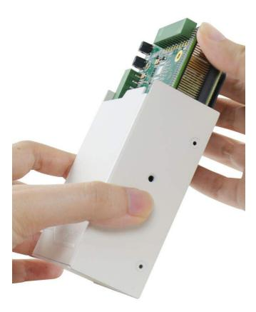
6. With the orientation shown below, gently press down and slide the holder in the direction shown to unclip the microSDHC card. Flip open the holder to install/ replace the microSDHC card.
