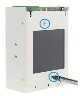
10. Install the cover, fasten the screws to secure the enclosure cover and cover plate.
