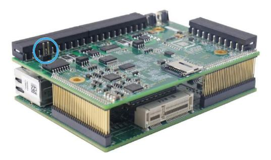
Jumper installed: resistance enabled
