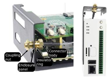
SMA female connector installation
