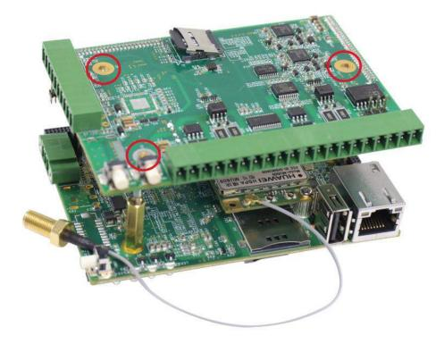
12. Insert the PCBA back into the enclosure, making sure the connectors\ buttons meet the enclosure openings and the SMA female connector is accessible.
