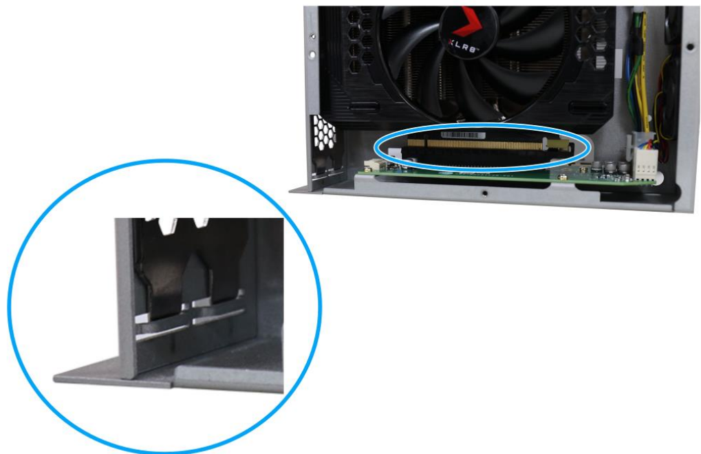
Make sure the card is inserted into the notch and PCIe slot
