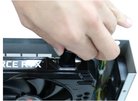
Connect the 8-pin power cable
