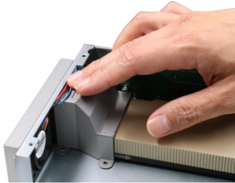
Reinstall the duct
