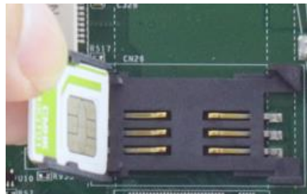
Insert Mini-SIM card with pins facing up
