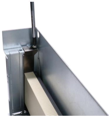
Remove the screws securing the graphics card
