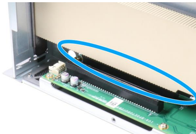
Properly inserted into the PCIe slot
