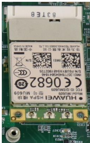
Insert on 45 degree angle
