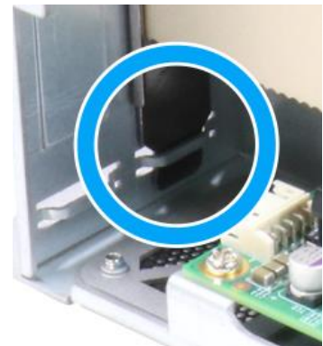
Bezel inserted into the notch
