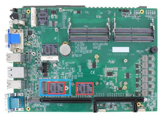
Before installing the mPCle module, you need to insert the Mini-SIM card. Slide the SIM slot holder and lift the SIM card holder. Insert the Mini-SIM card (pins facing up), shut the SIM holder and slide it to lock the SIM card in-place.
