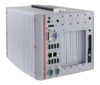
PCle slots (4-lanes) for expansion cards to extend function sets, making it that much more flexible for specific applications such as data collection, analytics and communication.
