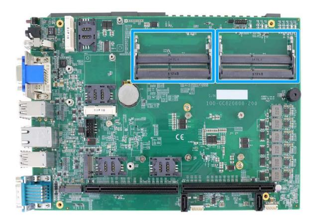
The system motherboard supports four 260-pin SODIMM socket for installing DDR4 memory module up to 128GB. Each slot supports single module DDR4 2133MHz SODIMM up to 32GB capacity.
