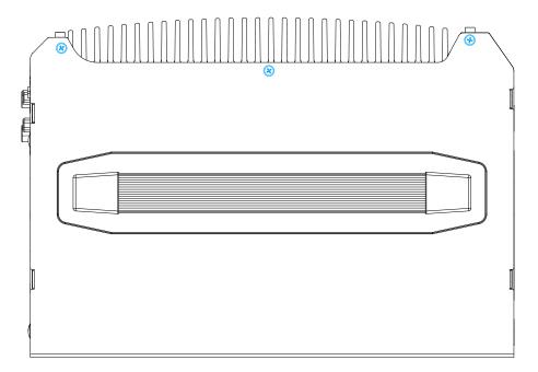
5. Secure the screws indicated in **blue** on the fan intake panel.
