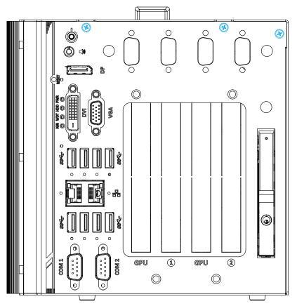
2. Remove the screws indicated in blue on the side panel.
