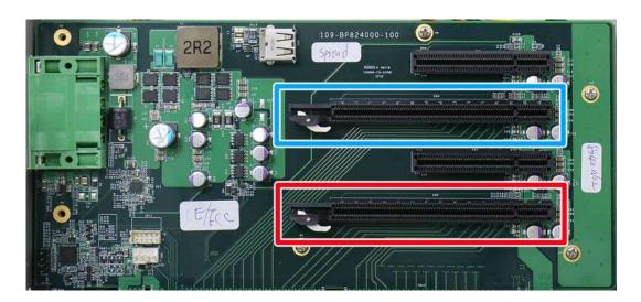
3. Remove the corresponding enclosure bezel(s) to the PCle slot you wish to install to .
