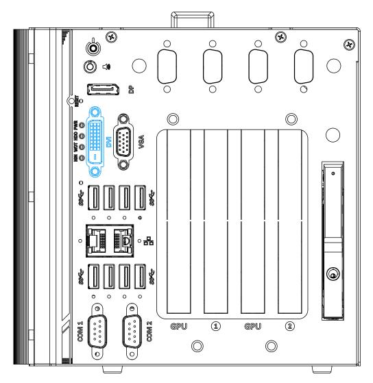
DVI-D transmits graphics data in digital format and therefore can deliver better image quality at high resolution. The DVI connector on the front panel can either output DVI signals or other digital signals (via an adapter/ cable) depending on the display device connected. It supports resolutions up to 1920x1200@60Hz.
