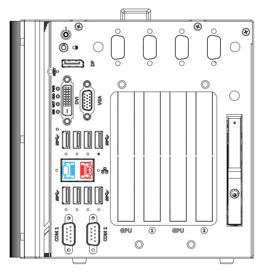
The system offers 2 GbE ports on its I/O panel. The GbE ports are marked in blue/ red and are implemented with Intel® I219-LM/ Intel® I210-IT controllers, respectively. Each port has one dedicated PCI Express link for maximum performance. When an Ethernet connection is established, the LED indicators on the RJ45 connector represents the following connection statuses:
