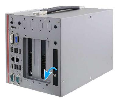
2. With the label side facing upward, insert the SATA connector side of the 2.5" HDD/ SSD into the slot first. You may feel resistance when the SATA connectors meet, push it firmly until the 2.5" HDD/ SSD is fully inserted into the slot.
