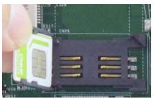
Insert Mini-SIM card with pins facing up
