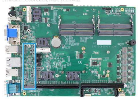
3. Insert the module on a 45 degree angle.
