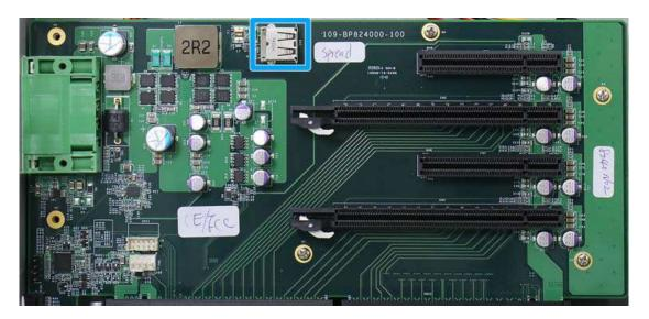
The system's daughter board has an internal USB2.0 port on the PCBA. You can utilize this USB port to connect a USB protection dongle inside the chassis of the system.
