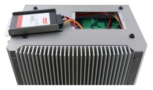
5. Tuck the cables into the enclosure, secure the HDD/ SSD and tray back into the enclosure.
