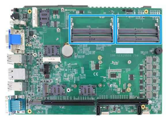
3. To install the memory module, insert gold fingers into the slot at 45-degree angle, push down on the memory module to clip the module into position.
