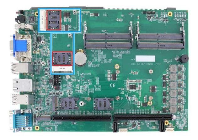
The system provides a dual mode mSATA/ mini-PCIe socket (indicated in blue) that is in compliance with mini-PCIe specification rev. 1.2. You can install either an mSATA SSD or mini-PCIe module into this socket and the system will automatically detect and configure it to run PCIe or SATA signals. This mini-PCIe socket is designed with SIM card (slot indicated in red) support. With a SIM card installed, your system can access the internet via your network provider's 3G/4G network.
