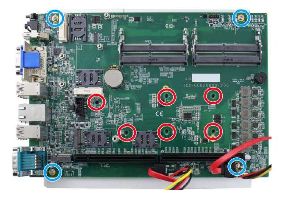
4. Gently separate the motherboard from the heatsink, you'll see the CPU socket protective cover, place finger tips underneath the sign "REMOVE" for leverage and gently lift the cover.
