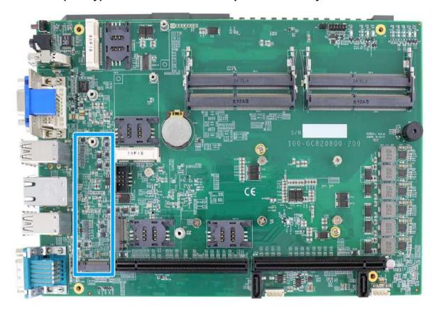
The system has anx4 PCIe M.2 2280 slot (also in compliance with SATA signal) for you to install an NVMe SSD for the ultimate performance or an Intel® Optane<sup>TM</sup> memory to accelerate the read/ write performances of traditional hard disk drive. An NVMe SSD offers exceptional performance over 2.5" SSDs while Intel® Optane<sup>TM</sup> memory can dramatically boost your traditional hard disk drives' read/ write performances.
