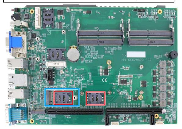
The system has an M.2 2242 slot (indicated in blue) that works with dual SIM slots (4G + 3G) on the front panel (indicated in red). By installing a 3G or 4G M.2 module and SIM card, you can access the internet via the provider's network.
