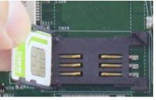
Insert Mini-SIM card with pins facing up
