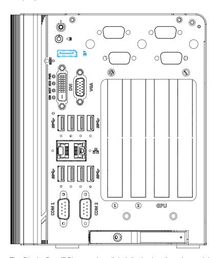
The DisplayPort (DP) output is a digital display interface that mainly connect video source and carry audio to a display device. When connecting a DP, it can deliver up to 4K UHD (4096 x 2304) in resolution. The system is designed to support passive DP adapter/ cable. You can connect to other display devices using DP-to-HDMI cable or DP-to-DVI cable.
