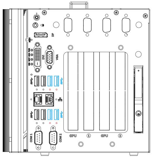
The system's USB 3.0 Gen 1 ports (5Gbps) are implemented via native xHCI (eXtensible Host Controller Interface) controller and are backward compatible with USB 2.0, USB 1.1 and USB 1.0 devices. Legacy USB is also supported so you can use USB keyboard/mouse in DOS environment. There are also screw-lock openings (indicated in red) for each USB port. xHCI driver is supported natively in Windows 10, therefore you do not need to install xHCI driver in prior to utilize USB functions.
