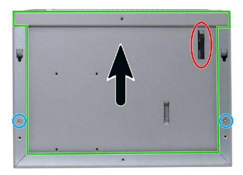
6. With the panel removed, you can now remove the extension board by removing the screws indicated in blue.
