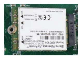
6. Gently press down and secure the module with an M2.5 P-head screw.
