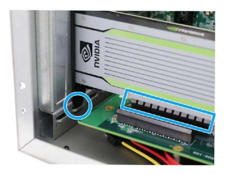
5. Secure the inference accelerator's bezel.
