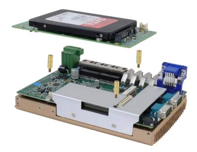
4. Then secure the  $MezIO^{TM}$  module to the hex bolts with three (3) P-head screws.
