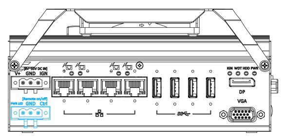
The "Remote On/ Off" 3-pin connection allows for external switch extension. It is useful when the system is placed in a cabinet or a not easily accessed location. You may connect an external remote with an external status LED indicator (15mA) by connecting to PWR LED and GND.
