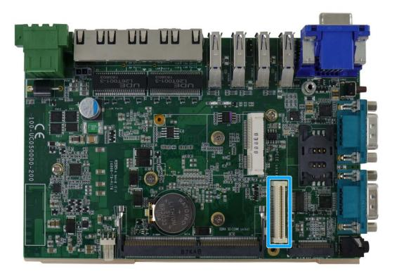
MezIO<sup>™</sup> is an innovative interface designed for integrating application-oriented I/O functions into an embedded system. It offers computer signals, power rails and control signals via a high-speed connector. MezIO<sup>™</sup> is also mechanically reliable benefited from its 3-point mounted mezzanine structure. A MezIO<sup>™</sup> module can leverage these signals to implement comprehensive I/O functions.
