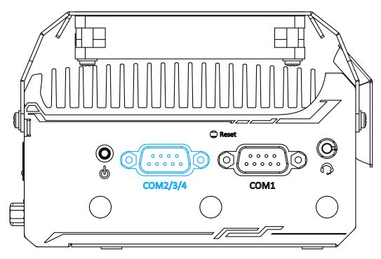
Implemented using industrial-grade ITE8786 Super IO chip (-40 to 85°C) and provide up to 921600 bps baud rate, the D-Sub male connector (COM2/ 3/ 4) can be configured in the BIOS as single RS-422/ 485 port (COM2) or three 3-wire RS-232 ports (COM2/COM3/COM4). Please refer to <u>COM2/ 3/ 4 Port Configuration</u> for configuring operation mode. An optional 1-to-3 Y-cable is available to connect three RS-232 devices.
