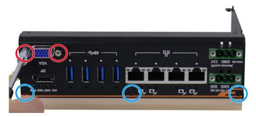
7. Unscrew the two (2) screws (indicated in red) to remove the DRAM/ NVMe SSD heat spreader and unscrew the screw (indicated in blue) to remove the DIO panel.
