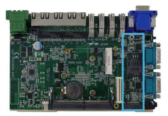
The system has an M.2 2280 slot (M key PCIe Gen3 x2) to install an NVMe SSD for the ultimate disk read/ write performance. An NVMe SSD offers doubled the disk read/ write speed performances over 2.5" SSDs.
