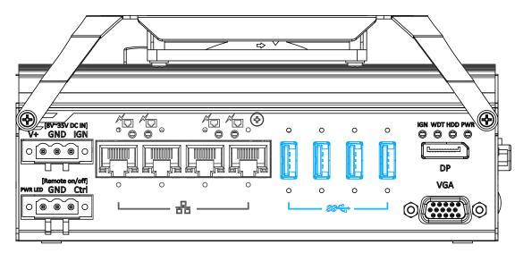
The system offers four USB 3.1 Gen1 (SuperSpeed USB) ports on its front panel. They are backward compatible with USB 2.0, USB 1.1 and USB 1.0 devices. Legacy USB support is also provided so you can use USB keyboard/mouse in DOS environment while USB 3.1 Gen1 driver is supported natively in Windows 10.
