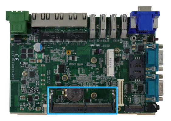
The system supports one 260-pin SO-DIMM socket for installing DDR4 memory module up to 16GB in capacity. Please refer to the following table for details.
