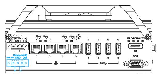
2. Connect the non-latched switch to the Remote On/ Off plug.
