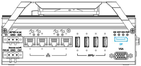
The system has a DisplayPort (DP) output which is a digital display interface that mainly connect video source and carry audio to a display device. When connecting a DP, it can deliver up to 4K UHD (4096 x 2160 @ 30Hz) in resolution. The system is designed to support passive DP adapter/ cable. You can connect to other display devices using DP-to-HDMI cable or DP-to-DVI cable.
