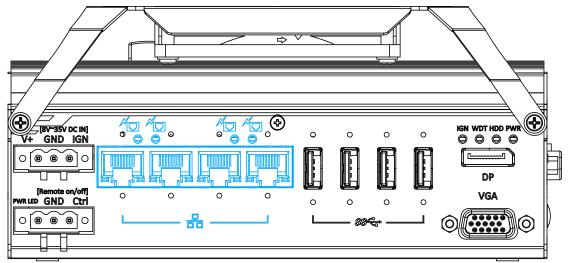
The Gigabit Power over Ethernet (PoE) port supply power and data on a standard CAT-5/CAT-6 Ethernet cable. Acting as a PSE (Power Sourcing Equipment), compliant with IEEE 802.3at, each port delivers up to 25W to a Powered Device (PD). PoE automatically detects and determine if the connected device is PoE PD or not before supplying power, making it compatible with standard Ethernet devices as well.
