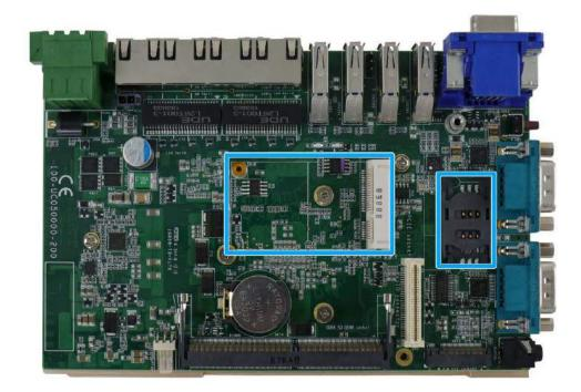
3. **To install**, insert mini-PCIe module's gold finger on a 45 degree angle into the socket, gently press the module down and secure it with a screw.
