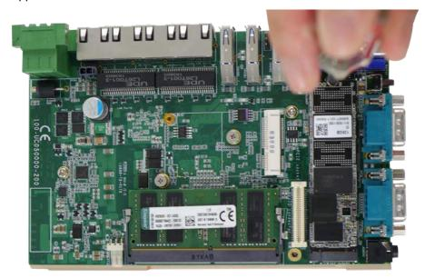
5. Once you have installed the NVMe SSD, you need to reinstall the heat spreader but before you do so, please make sure the protective film on the thermal pads have been removed.
