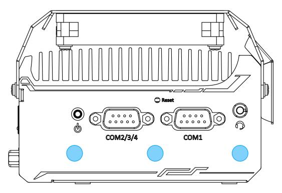
The system offers three SMA antenna openings reserved for SMA antenna installations. Users can take advantage of these three openings when installing mini-PCIe module for wireless communication reception such as 3G, 4G, GPS or WiFi.
