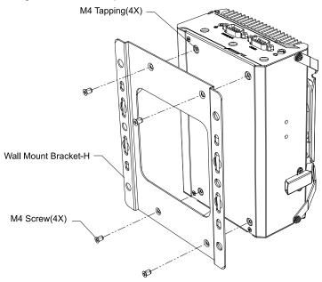
2. Dimension illustration of the install wall horizontal mount bracket for you reference.
