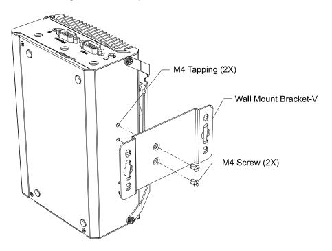
2. Dimension illustration of the install vertical wall mount bracket for you reference.
