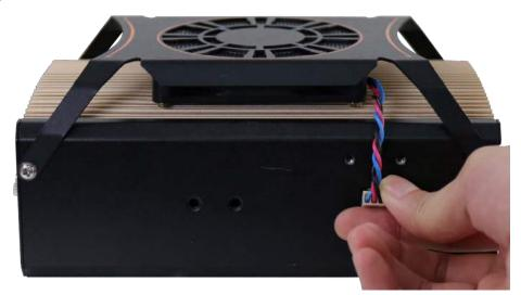
Plug in the 3-pin fan power connector
