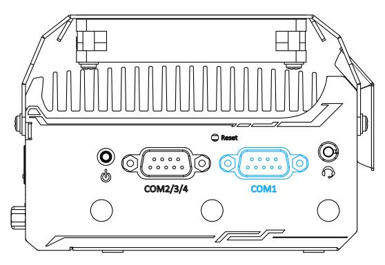
Implemented using industrial-grade ITE8786 Super IO chip (-40 to 85°C) and provide up to 921600 bps baud rate, COM1 is a software-configurable RS-232/422/485 port via 9-pin D-Sub male connector. The operation mode, slew rate and termination of COM1 can be set in BIOS setup utility. The following table describes the pin definition of COM ports.
