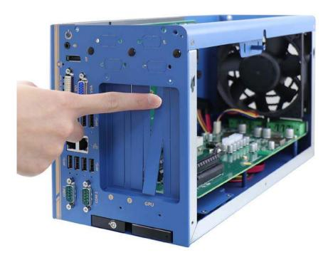
4. Remove the graphics card from the antistatic bag and gently lower it into the PCIe slot while ensuring the gold-fingers meet, graphics card panel is properly inserted and secured with screws.
