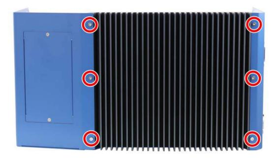
9. The system's internal I/Os are now accessible and the CPU is ready for installation once the motherboard is separated from the heatsink. Please refer to the CPU installation section on how to separate the motherboard from the heatsink.
