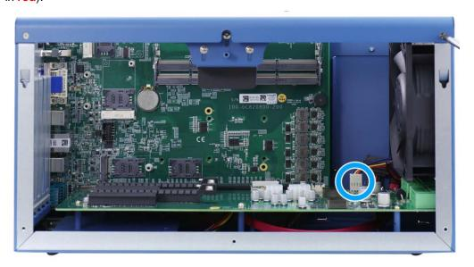
Remove 4-pin fan connector
