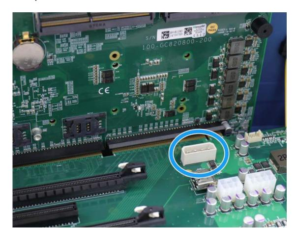
The 4-pin molex connector can be found on the extension board. It can provide additional power supply for power hungry add-on cards such as PCIe PoE cards. The pin definition are as follows:
