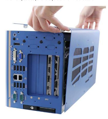
6. Once the L-shaped side panel has been removed, proceed to remove the graphics card's stabilizer plate by removing the three screws.
