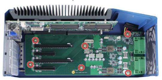
Remove screws to separate the extension board from the motherboard
