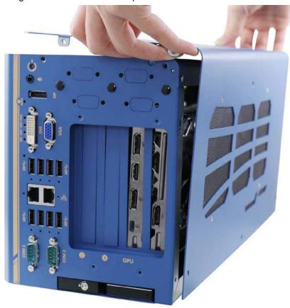
Place L-shape side panel onto the enclosure
