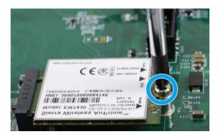
Clip on the IPEZ-to-SMA cable to the module and secure the antenna to the front or rear panel. Please refer to the module's manual for clip-on connection. If you need to install other components, please refer to respective sections.
