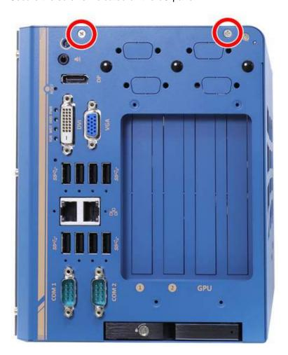
3. Secure the screw indicated on top of the enclosure.
