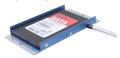
At the tray opening, you should be able to locate the 22-pin SATA cable, connect it to the installed HDD/ SSD. Due to cable length limitations, the connector side of the HDD or SSD should be facing towards the bottom of the enclosure.
