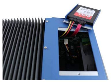
4. Insert the tray back into the system and secure it with two screws you removed earlier.
