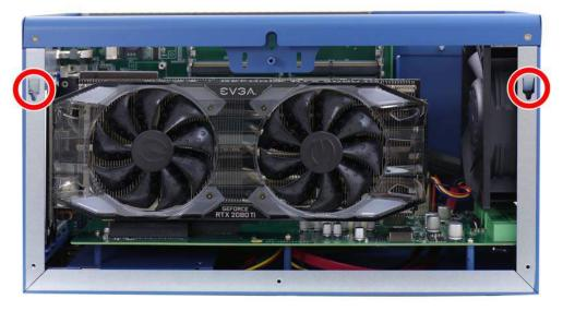
Slide-and-lock into the indicate hinges
