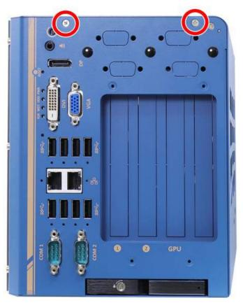
2. Unscrew the screw indicated on top of the enclosure.
