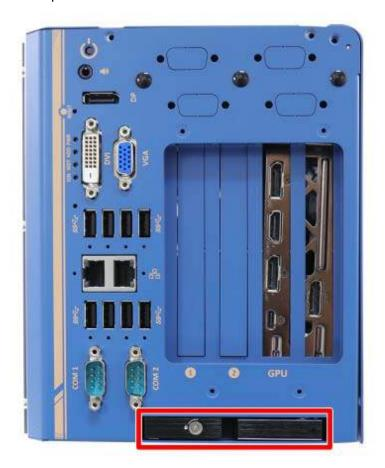
You may insert and install the HDD/ SSD without disassembling the enclosure. Simply lift to spring open the lever to gain access to the hot-swap slot.
